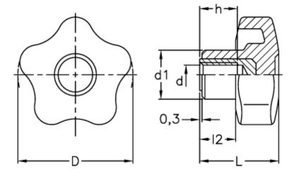
$$\begin{array}{ll} D & = 25 \\ d1 & = 13 \\ d \ 6H = M6 \\ h & = 10 \\ L & = 19 \\ l2 & = 8 \end{array}$$
